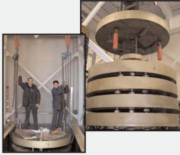
Or that one nick on the deadweight could mean a lost gram; and a 5-mile change in location means a change in gravity of 0.0009%?
